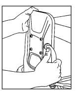
To adjust the mirrors when towing a trailer, turn the mirror by pushing the mirror head toward the front of the vehicle.
